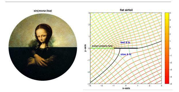
The image on the left is a graphical answer to the complex analysis question, "What is the sine of the Mona Lisa?". It is an example of a conformal map. The image on the right is a visualization of airflow past a flat airfoil (thick black) – the flow follows the orange curves in the direction from the lower left to the upper right. The curves are level contours obtained from a complex-valued function.
