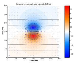
The image above shows the streamlines and wind vectors for a surface dipole from a model of atmospheric flow. The dipole is obtained as a solution to a three-dimensional Laplace PDE with mixed boundary conditions. Its computation involves a numerical implementation of an integral Hankel transform – an example of applied special function theory.
