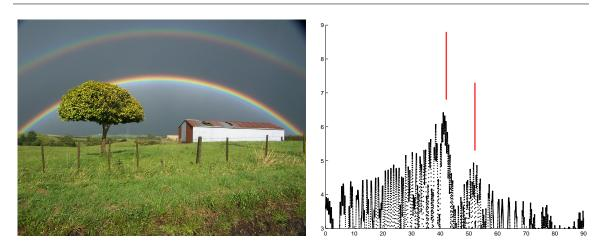
The image on the left shows the primary (lower) and secondary rainbows, with the so-called Alexander's dark band in between. The plot on the right shows backreflected light intensity (log-scale) versus viewing angle of a "separation of variables" rainbow computed using Bessel functions. This plot, based upon a solution of the Helmholtz PDE, predicts (noisy) intensity peaks very near the  $42^{\circ}$  and  $52^{\circ}$  angles (red lines) as observed for the familiar rainbows.
