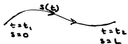
$$s = s(t) = \int_{t_1}^t \left| \frac{d\vec{R}}{dt} \right| dt \quad , \quad t \geq t_1$$
