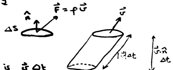
In time interval  $\Delta t$ , displacement is  $\vec{v} \Delta t$
