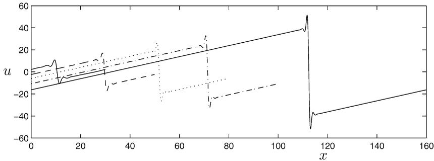
Fig. 3. Stationary viscous shock solutions for  $\varepsilon^2 = 1.5$ , and (from left to right, in increasing order of height) for  $L = 30$ ,  $L = 50$ ,  $L = 80$ ,  $L = 100$  and  $L = 160$  (here the periodic domain is taken as  $\Omega = [0, L]$ ).
