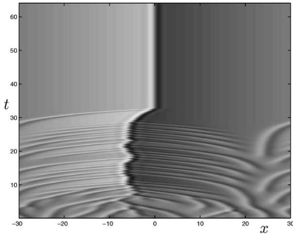
Fig. 1. Evolution of destabilized KS equation (3), with  $L = 60$  and  $\varepsilon^2 = 1.4$ , showing the rapid convergence to a stable shock-like solution; in this gray-scale representation of the space–time evolution, lighter shading indicates local maxima, darker shows minima, and the shading interpolates between extremes of  $u = \pm 25$ .
